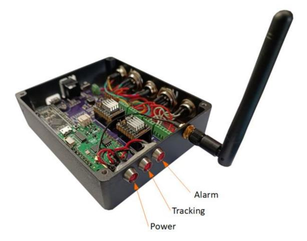
The LEDs are pretty self explanatory. Power will illuminate when you plug the mount in (ground breaking stuff!). The tracking LED is a good confirmation that the controller is working properly as the mount starts tracking when powered on & this LED will flash. If you have modified the firmware or applied one of our software updates and this LED is not flashing after a restart you have a clear indication that something went wrong. The alarm LED
